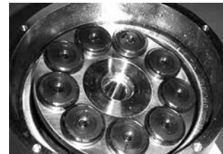
14. Place pistons in retaining plate and cylinder barrel. When pistons are placed, tilt retaining plate for easier placement of swash plate. If swash plate has been disassembled from mounting flange, see page 14 for assembly of swash plate. 15. Lubricate piston shoes and swash plate with clean filtered water. Remember to place the pins in housing.
