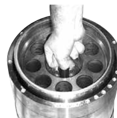
15. Mount a 8 mm eye bolt in the cylinder barrel. Pull straight upwards. A continuous lift will elevate the cylinder barrel out of housing. This can only be done if shaft seal is removed.
