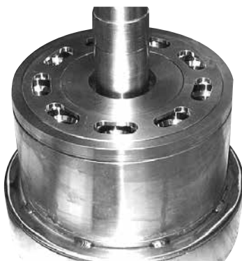
16. Place cylinder barrel upside down. For further disassembling of cylinder barrel and valve plate see page 11.
