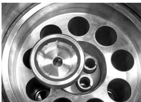
14. Remove the retainer guide, the 4 springs and the spring guide.
