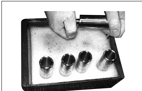
13. Place retaining guide, retaining ball and retaining plate in cylinder barrel. Note: If pistons are replaced, place new pistons in clean filtered water for a couple of minutes. Exercise piston shoes to make them "run" smoother.
