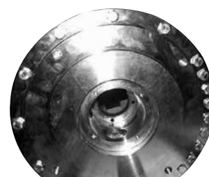
19. Place the pump horizontally. Remove the remaining screws in port flange by using a 13 mm combination wrench. Carefully separate house and port flange. Ensure that pin for the positioning house is not lost. For further disassembling of flush valve, see page 16.
