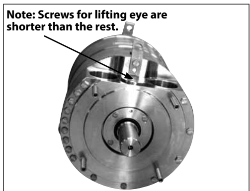
17. Screw in the rest of the bolts and cross tighten all screws to a torque of 30 +/- 2 Nm.
